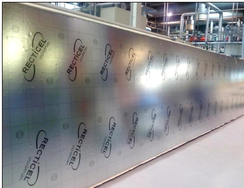
Figure 4: Picture of an insulation board produced during semi-industrial trials (width:1.2 m; length:6 m).
